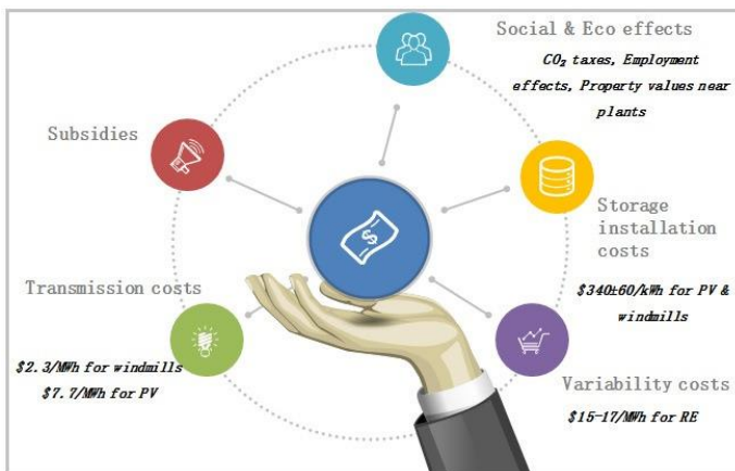
Figure 2 Parameters to be integrated in the calculation of the LCOE for a more realistic perspective
